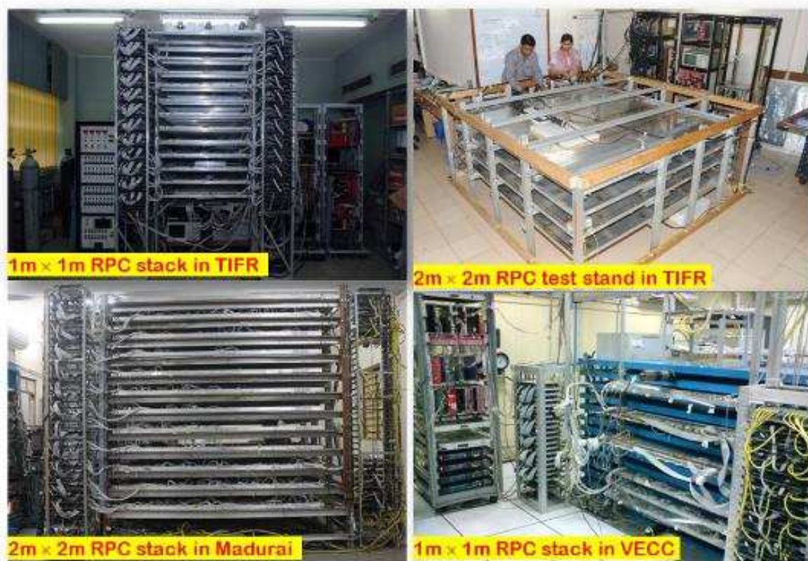
Figure 3: RPC test stands built at various INO labs and being operated round the clock for several years
