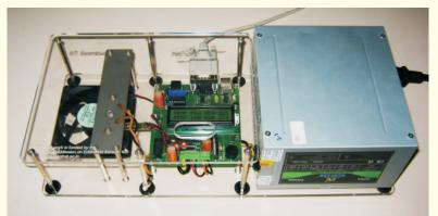
Figure 1: Single Board Heater System
